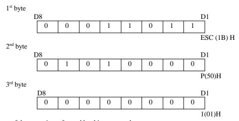
A partial cut of the paper is performed by this command.
